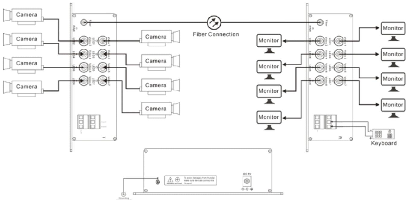
To install, connect the video inputs to the SWV60801-T, connect the video monitors or other video receptors to the SWV60801-R, and connect an appropriate optical fiber between the SWV60801-T and SWV60801-R optical ports. Connect data signal sources or destinations, as required, to the "DATA" port per the following Built-In Data Connection section.
